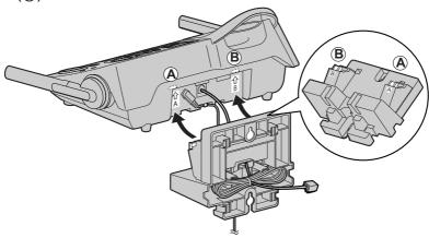
**4** Adjust the adaptor to hold the base unit, then push it in the direction of the arrow until it clicks into place.
